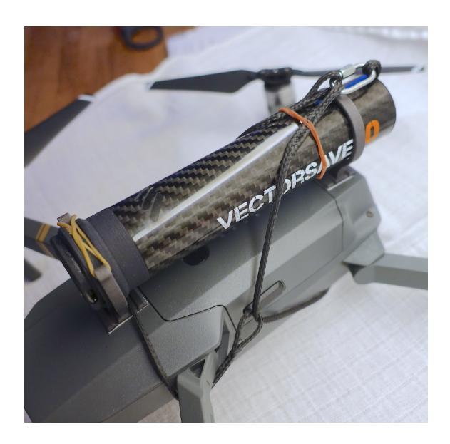
Mavic battery can be changed by lifting front part of the tube from clip. No need to take away the whole setup. Harness can be left on for transportation too. Mavic will fold nicely with the harness in place.
